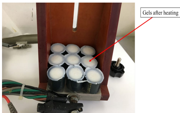
Fig. 3. Surimi gels prepared by ohmic heating.
